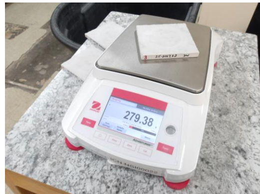
Photo No. 4 ASTM C1353 – Representative Post- Abrasion Mass Determination
