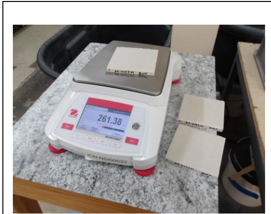
Photo No. 1 ASTM C1353 – Pre-Abrasion Specimen Mass Determination
