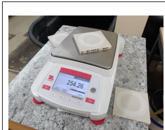
Photo No. 4 ASTM C1353 – Representative Post- Abrasion Mass Determination
