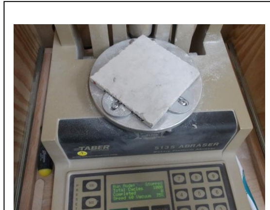
Photo No. 2 ASTM C1353 – Abrasion Apparatus and Pretest Specimen Condition
