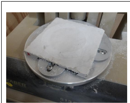
Photo No. 3 ASTM C1353 – Representative Post- Abrasion Specimen Condition
