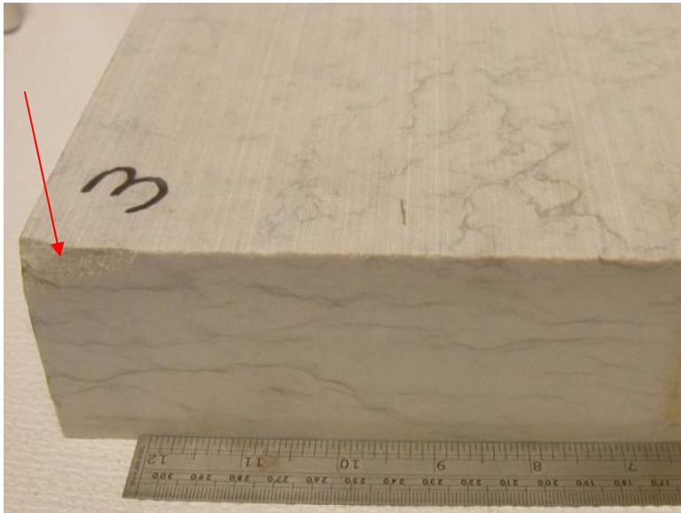
Figure 7. Slab 3 - Oblique view of corner showing minor chip (arrow) attributed to handling damage.
