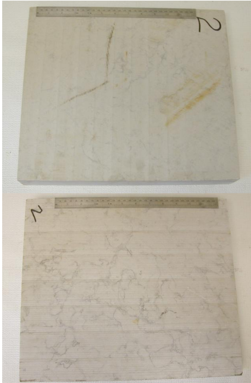
Figure 2. Slab 2 - Top and bottom surfaces at completion of FT testing.
