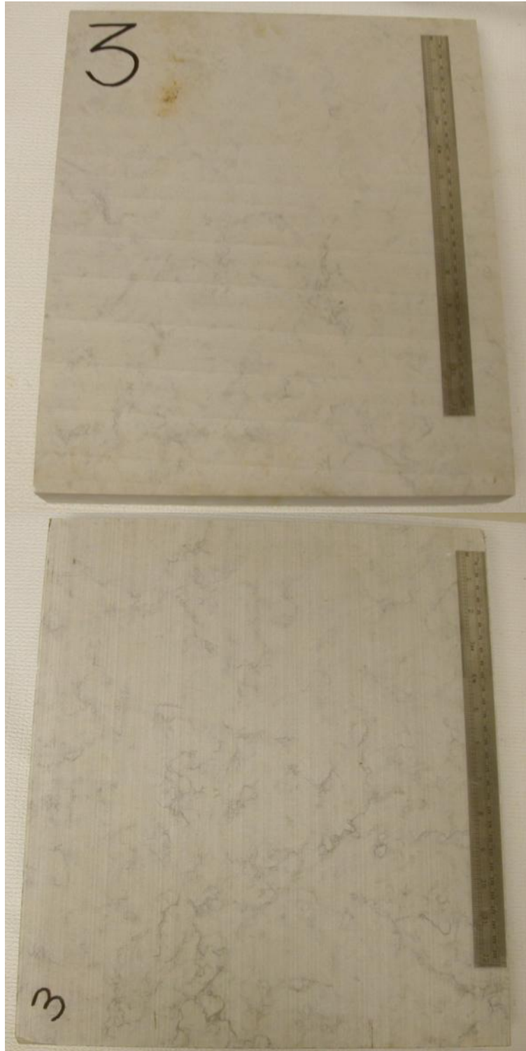
Figure 3. Slab 3 - Top and bottom surfaces at completion of FT testing.
